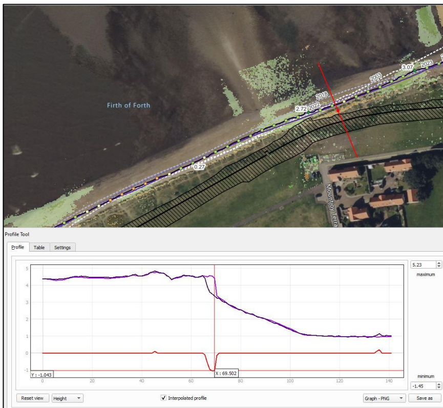
Figure 23: Pre- and post-Storm Babet height and MHWs changes at the proposed easterly hybrid defence structure (hatched black), showing two surface elevations in cross-section (pink pre-Babet, purple post-Babet, nett vertical change in red). The red dot on the map along the red cross-section line between the structure (hatched) and the various MHWs lines indicates the position (at 69.502m from start of cross-section) on the cross-section diagram.
